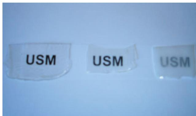
**Figure 11** Images of films (400–600  $\mu\text{m}$ ) of PMMA (left one), PMMA-Lap-MPTS-CTAB (middle image), and PMMA-Lap-MPTS (right image). [Color figure can be viewed in the online issue, which is available at [www.interscience.wiley.com](http://www.interscience.wiley.com).]
